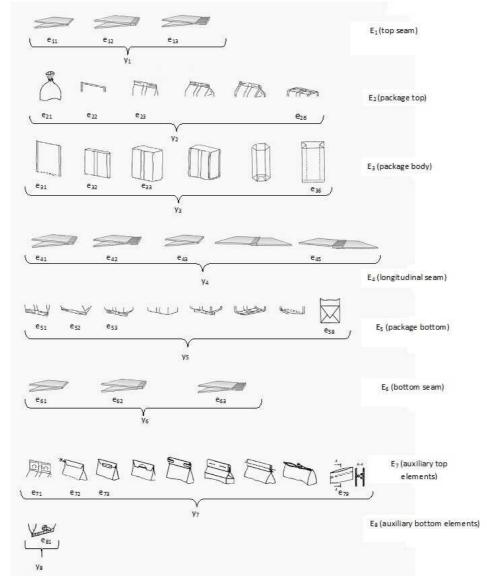
Fig. 1. Family of the elements of package
