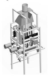
Fig. 4. 3D model of the designed versatile packaging machine
