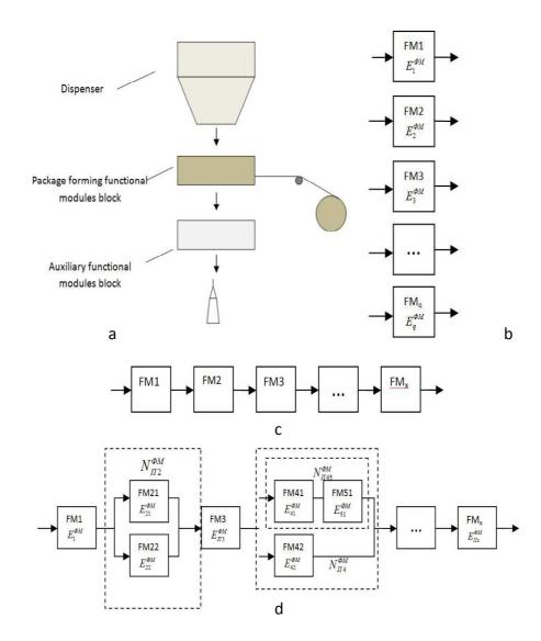
Fig. 2. General structure of the packaging machine (a) and the schemes of the parallel (b), serial (c) and mixed (d) connection of FMs
